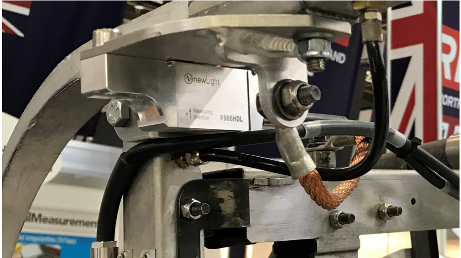
Fig. 3.5 Mounted FS66HDL Force Sensor on a pantograph
