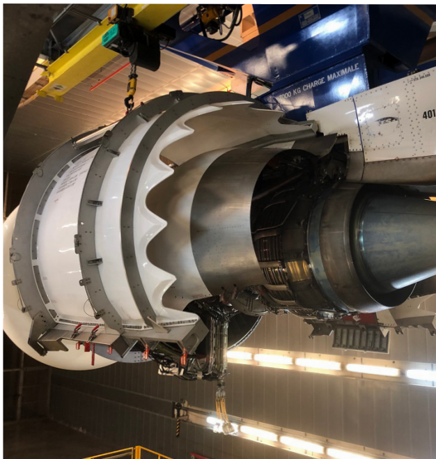
Engine mounted inside a test cell for performance validation
