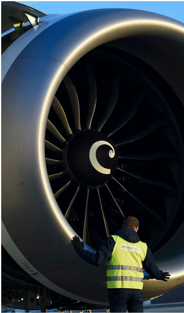
Visual inspection of a nacelle
