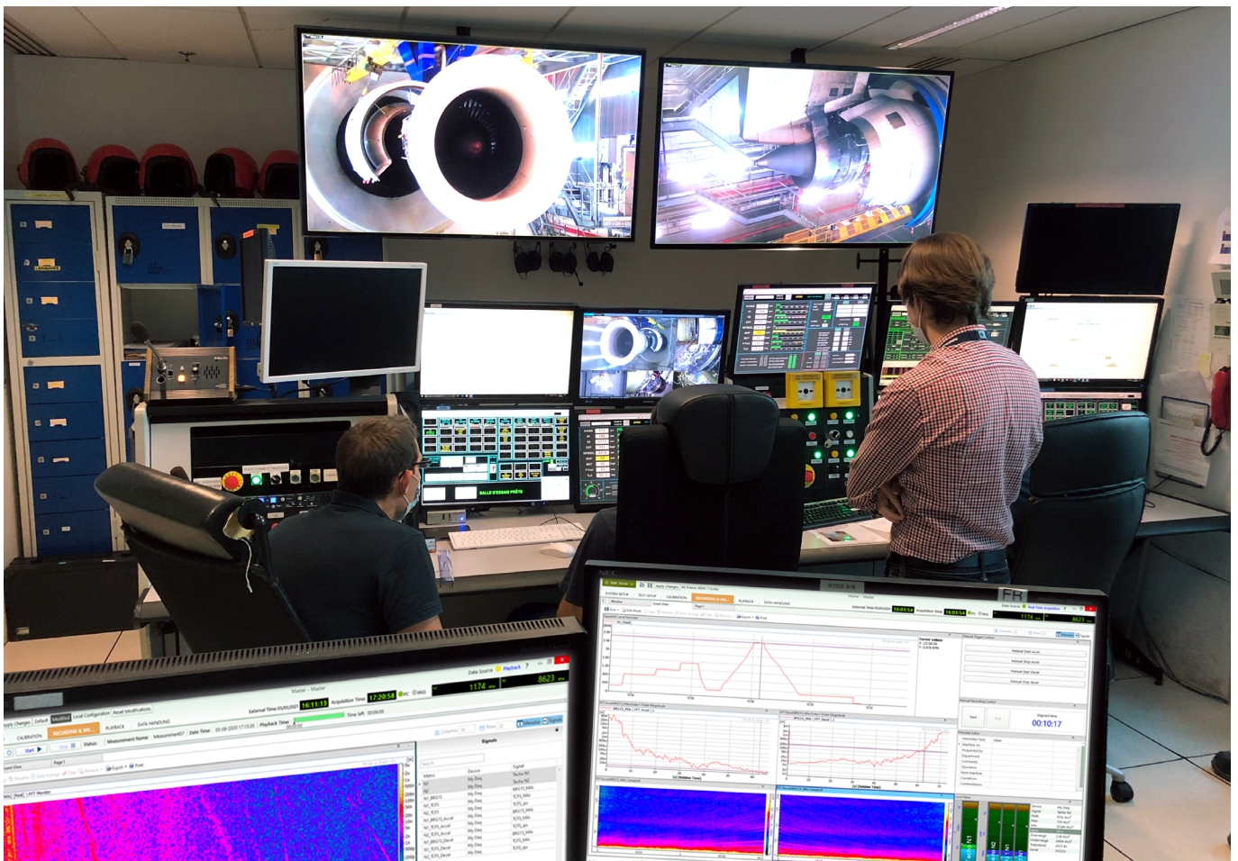
A performance test seen from inside the control room, with Tescia software providing additional data insight and validation
